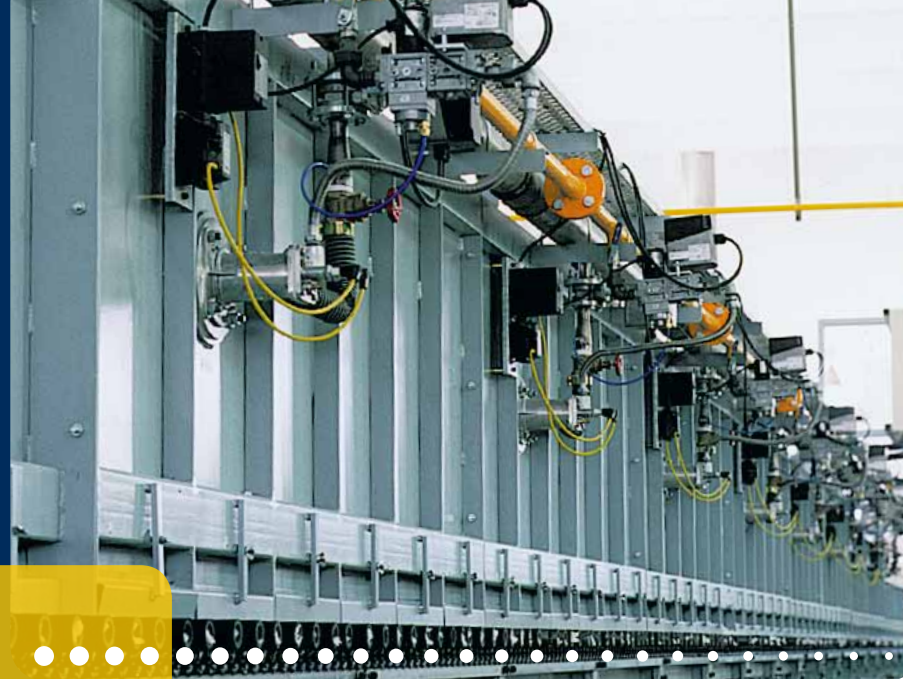
Roller hearth kiln, works photograph Dum-Kilnogy S.A.
