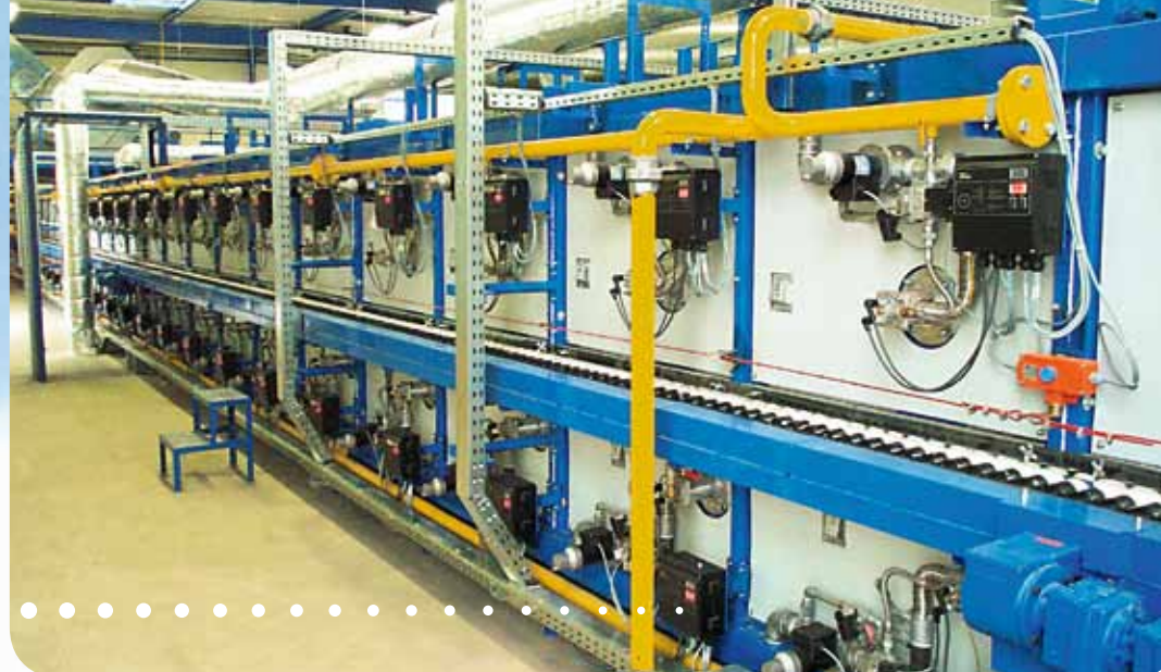
Roller hearth kiln, works photograph Laeis Bucher
