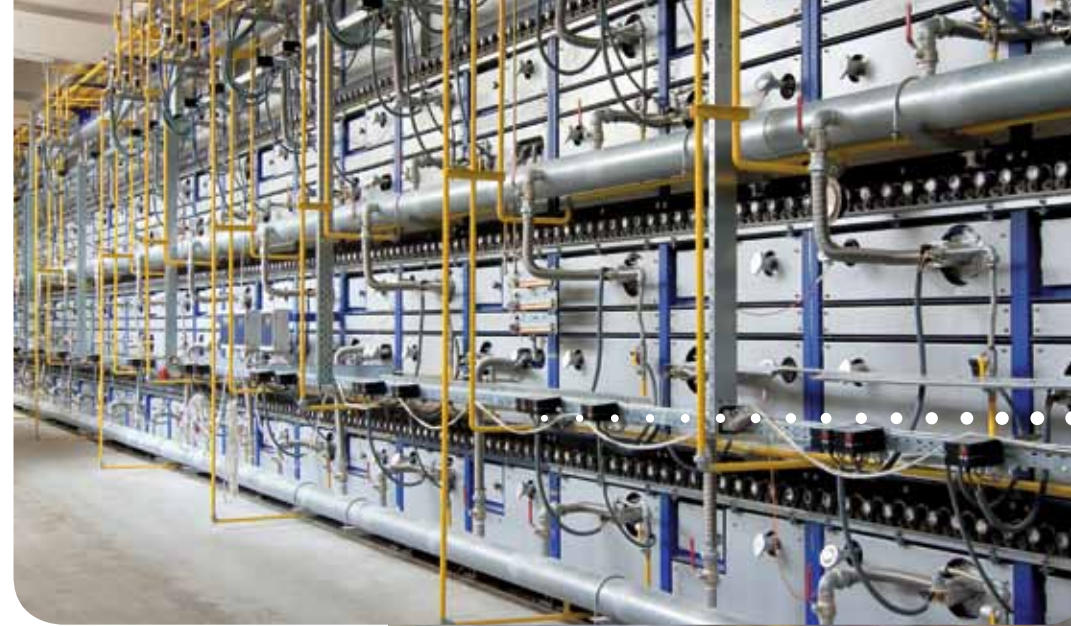
Roller hearth kiln, works photograph Laeis Bucher
