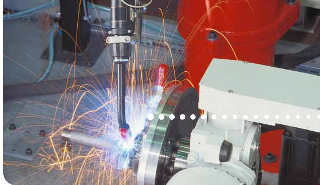
Welding robot for burner production
