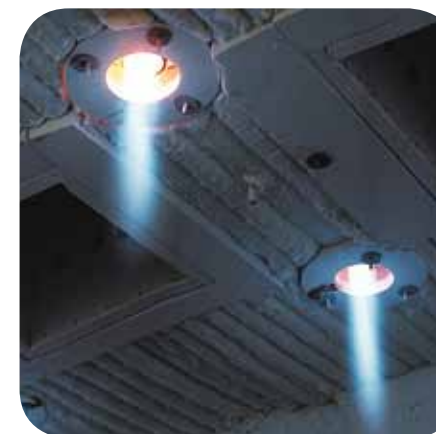
Overhead firing with BIC burners
