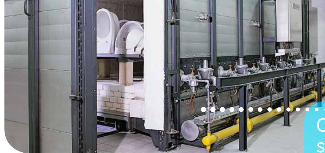
Intermittent shuttle kiln, works photograph Eisenmann
