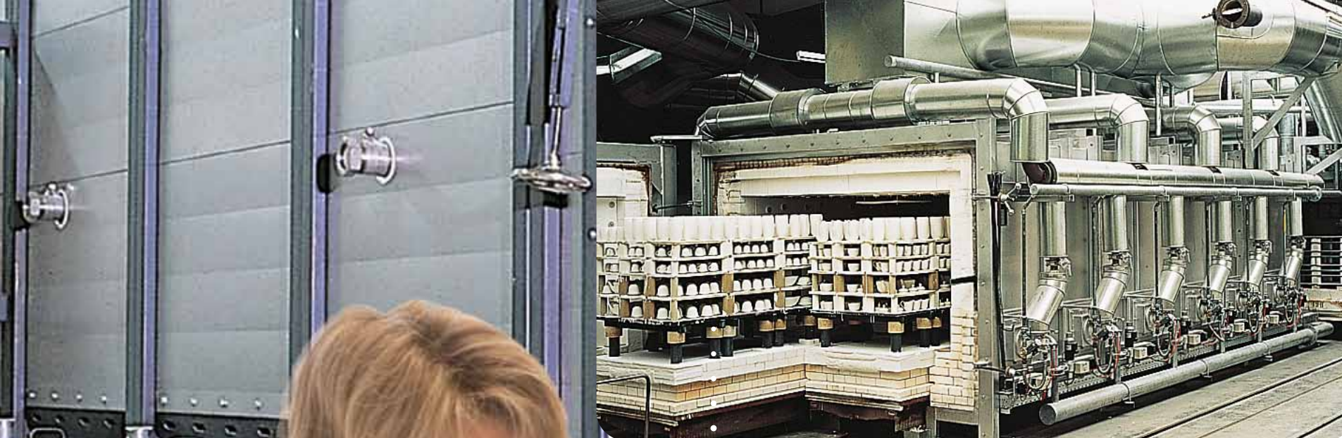
Roller hearth kiln, works photograph Riedhammer
